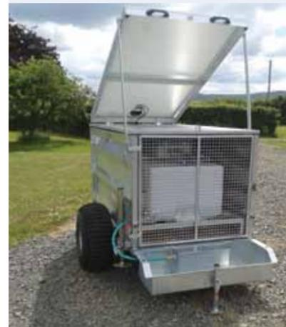
The portable solar powered water system developed by Cheviot Futures and Inherent Energy in partnership with the farm business at West Fenton, July 2013. Rear view showing the holding tank and inclusive trough arrangement.
