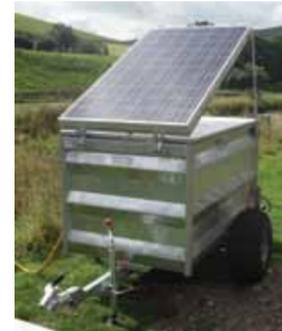
*The innovative prototype trailer mounted solar PV alternative watering system*
