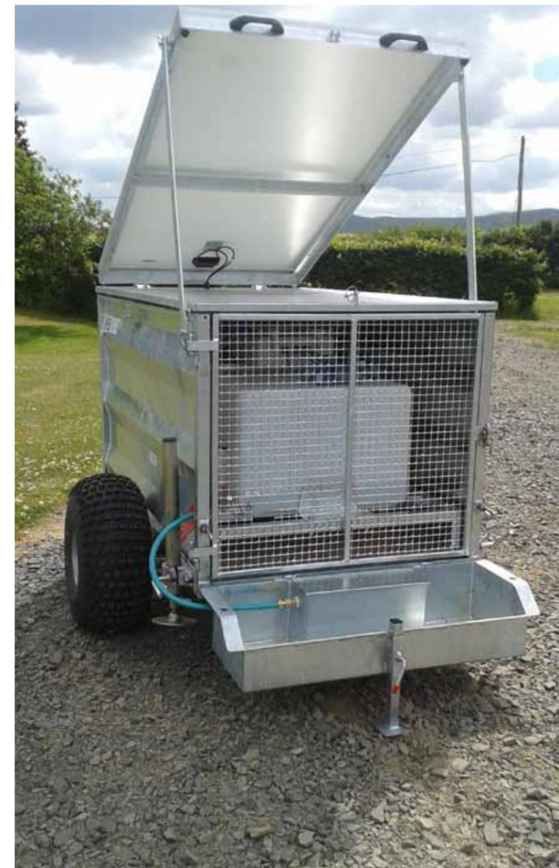
The portable solar powered water system developed by Cheviot Futures and Inherent Energy in partnership with the farm business at West Fenton, July 2013. Rear view showing the holding tank and inclusive trough arrangement.
